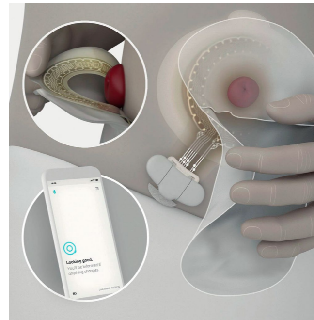
Figure 1: The Heylo system comprises a sensor layer to be applied underneath the user's baseplate. The sensor layer continuously monitors for moisture between the skin and baseplate, and the status of the baseplate is conveyed to the user via a Bluetooth transmitter to an application on a smartphone. The transmitter charger is not shown here. The user has access to technical support when needed.
